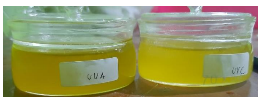
Figure 2. The results of irradiating cooking oil using UV-A and UV-C rays at a maximum photooxidation of 12 hours
