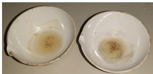
Figure 5. the results of oil samples at a temperature of 110 °C. there is a black precipitate in the middle of the sample which is the powder of the charred leaves of the tapak dara due to heating
