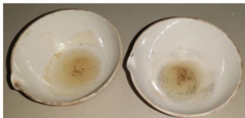
Figure 5. the results of oil samples at a temperature of 110 °C. there is a black precipitate in the middle of the sample which is the powder of the charred leaves of the tapak dara due to heating
