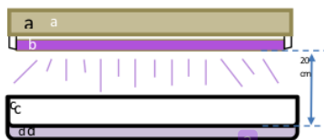
Figure 1. Ultraviolet photooxidation design. (a). ballast, (b)UV-C/A tube lamp, (c) sample container, (d) test oil
